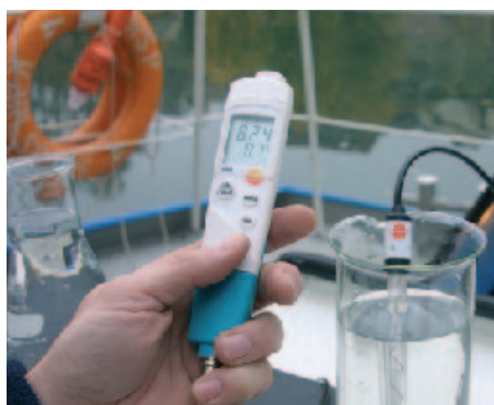
Automatic temperature compensation in external probes with temperature sensor
