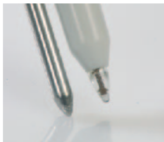
pH tip embedded in break-proof plastic
