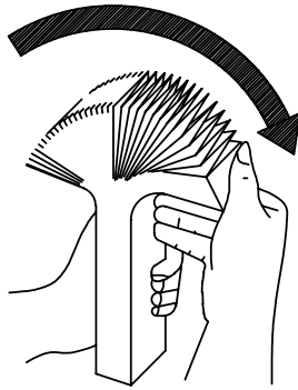
Fig. 5.1-5 Loosening the Chart Paper
