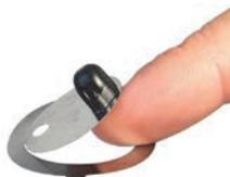
Since the diaphragm only bends, and functions without a bearing, there is almost no frictional effect and extremely little wear. The movement occurs practically free of hysteresis, and the test results have very good reproducibility. The diaphragms low bulk results in a rapid response time. The almost complete covering of the flow cross-section in the neutral position enables a very low metering range start value.
